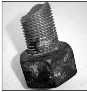
Photo #4--Bolt severed by high pressure.
